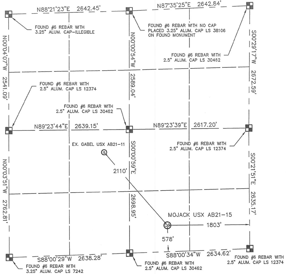
In accordance with a request from ERIK VAN DECAR with NOBLE ENERGY INC. King Surveyors Inc. has determined the surface location of the MOJACK USX AB21-15 to be 578' from the SOUTH line and 1803' from the EAST line, as measured at right angles, from the section lines of Section 21, Township 7 North, Range 64 West of the Sixth Principal Meridian, County of Weld, State of Colorado.
