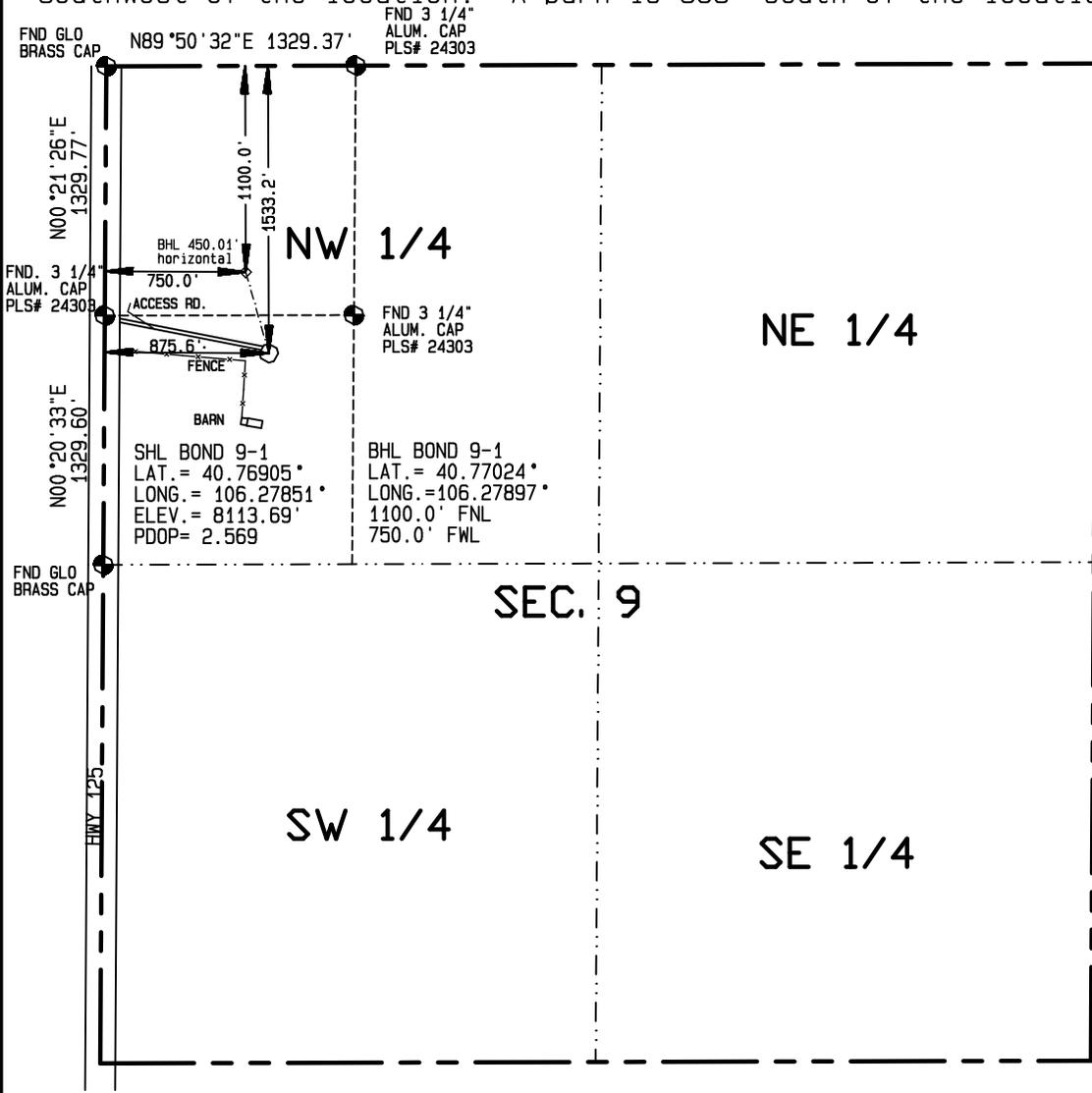
BASIS OF BEARINGS IS THE NORTH LINE OF THE NW1/4 NW 1/4 OF SEC. 9, T9N, R79W OF THE 6TH P.M. JACKSON COUNTY, CO. BEARS N89°50'32"E BETWEEN SET MONUMENTS AS DETERMINED BY GPS (NAD 83)
