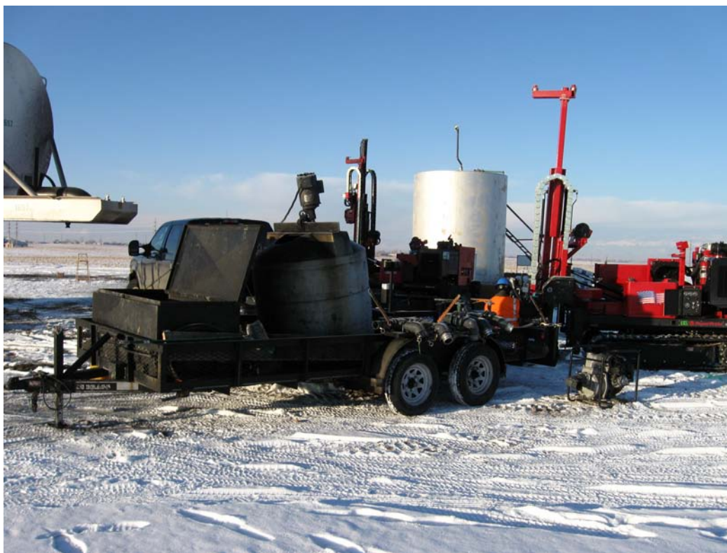
Photograph 2: Carbon slurry mixing equipment.
