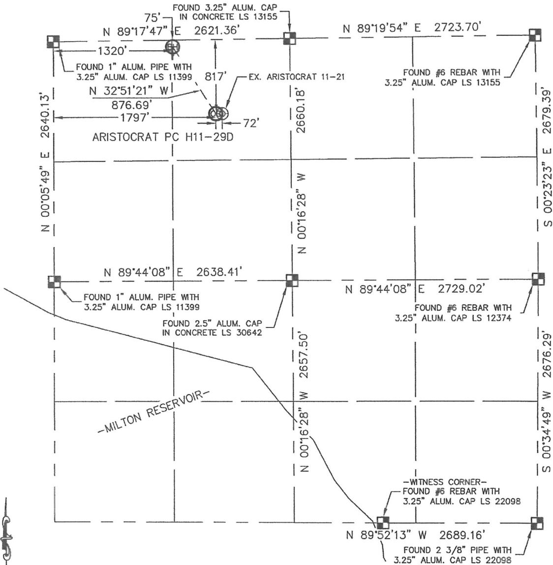
In accordance with a request from Erik Van Decar with Noble Energy Inc. Lat40°, LLC has determined the surface location of the ARISTOCRAT PC H11-29D to be 817' from the NORTH line and 1797' from the WEST line and the bottom hole to be 75' from the NORTH line and 1320' from the WEST line as measured at right angles from the section line of Section 11, Township 3 North, Range 65 West of the Sixth Principal Meridian, County of Weld, State of Colorado.
