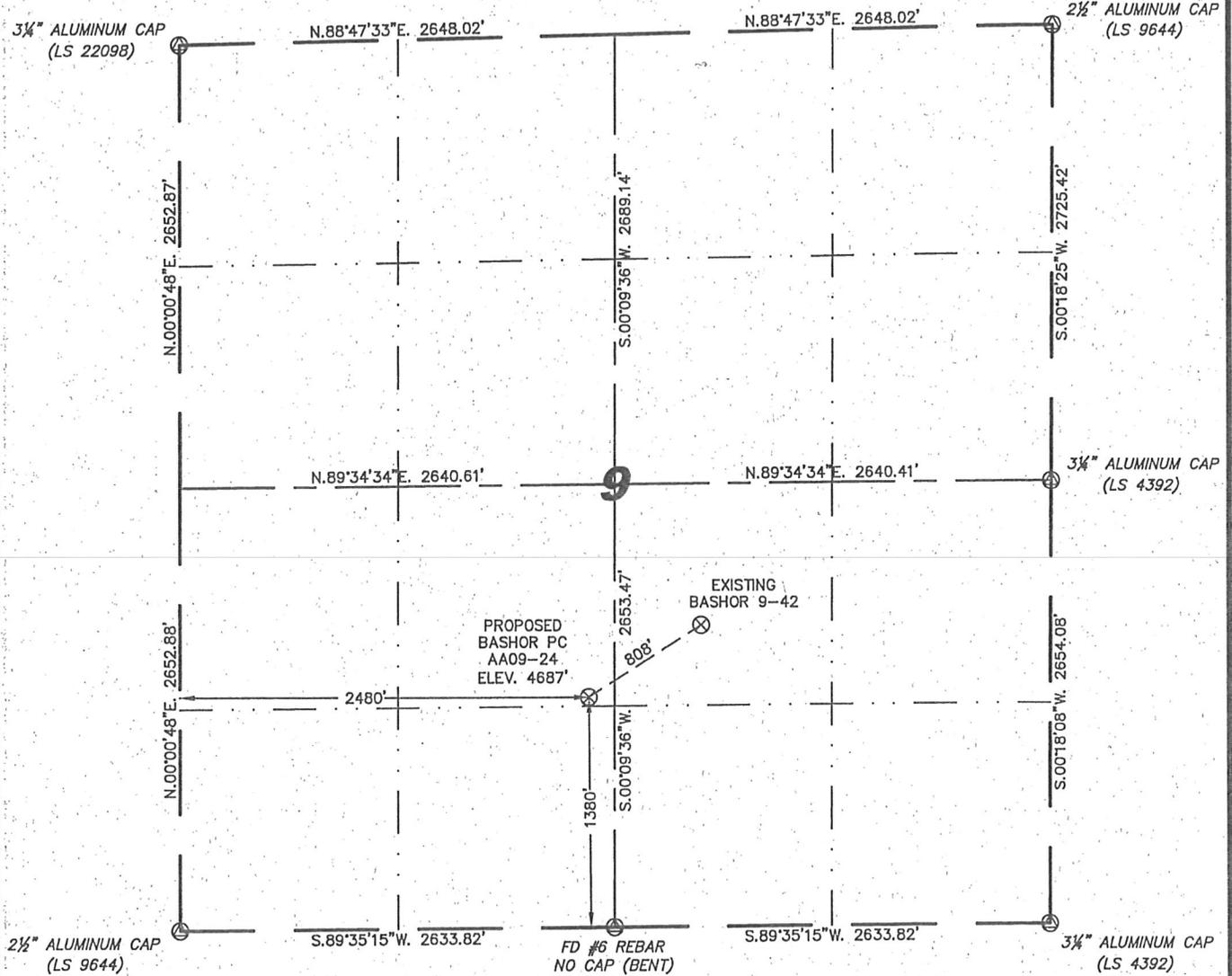
IN ACCORDANCE WITH A REQUEST FROM ERIK VAN DECAR - NOBLE ENERGY INC, STEIL SURVEYING SERVICES, LLC HAS DETERMINED THE LOCATION OF THE BASHOR PC AA09-24 WELL TO BE 1380' FSL, 2480' FWL, AS MEASURED AT NINETY (90) DEGREES FROM THE SECTION LINES, SECTION 9, TOWNSHIP 6 NORTH, RANGE 63 WEST, 6TH PRINCIPLE MERIDIAN, WELD COUNTY, COLORADO.
