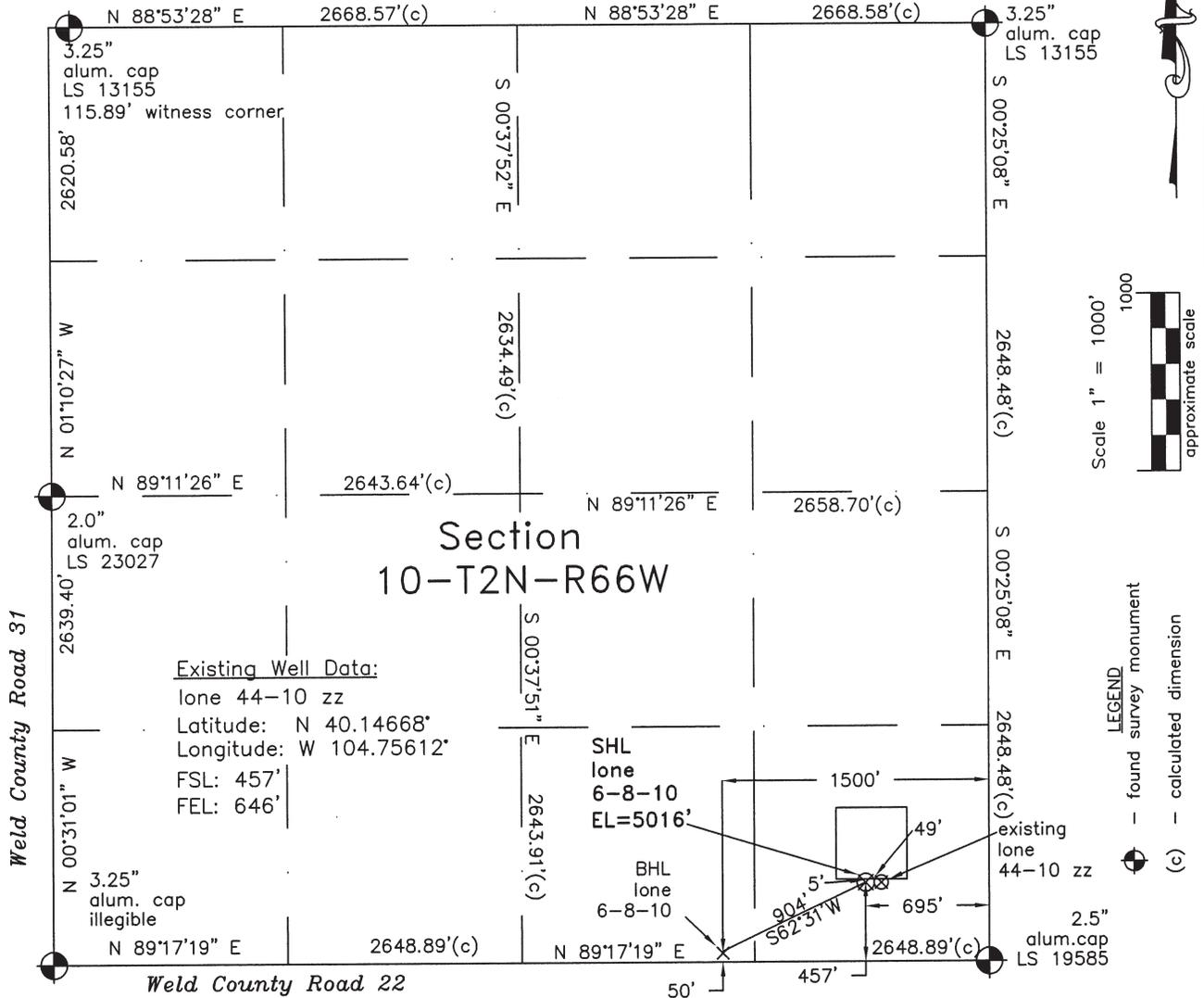
In accordance with a request from Dave Bale of EnCana Oil & Gas (USA) Inc., Frederick Land Surveying, Inc. has determined the location of the **lone 6-8-10** well site to be SHL: 457' FSL and 695' FEL, BHL (50' FSL and 1500' FEL) as measured at ninety (90) degrees from the section lines of Section 10, Township 2 North, Range 66 West, 6th Principal Meridian, Weld County, CO.
