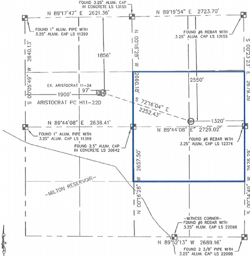
In accordance with a request from Erik Van Decar with Noble Energy Inc. Lat40°, LLC has determined the surface location of the ARISTOCRAT PC H11-22D to be 1856' from the NORTH line and 1900' from the WEST line and the bottom hole to be 2550' from the NORTH line and 1320' from the EAST line as measured at right angles from the section line of Section 11, Township 3 North, Range 65 West of the Sixth Principal Meridian, County of Weld, State of Colorado.
