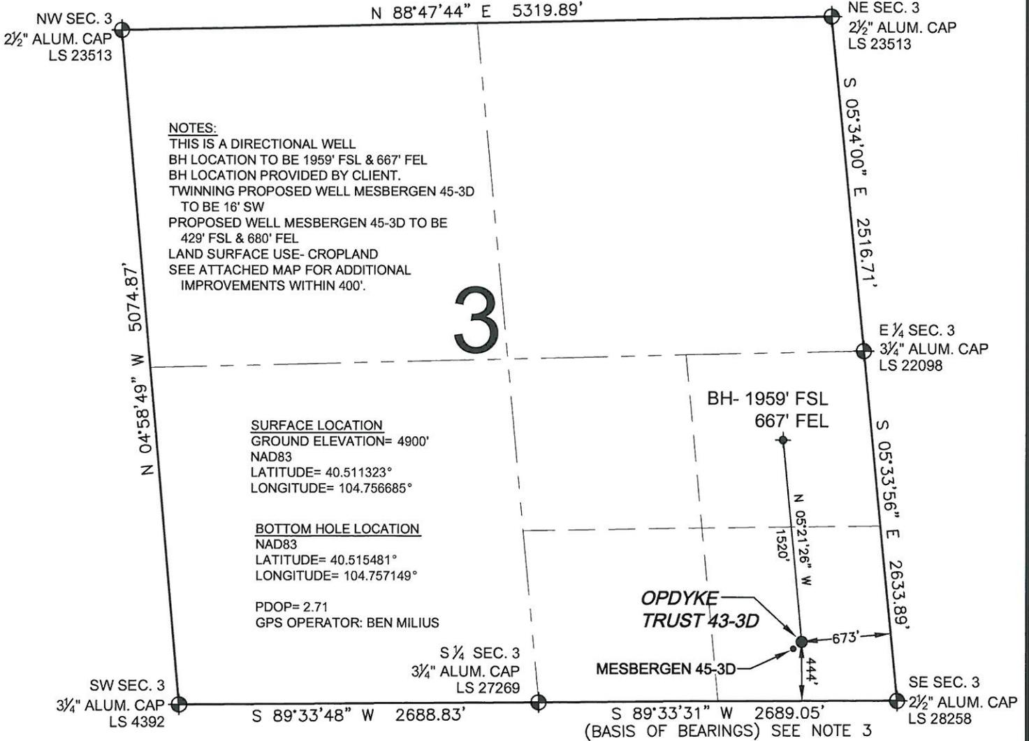
WELL **OPDYKE TRUST 43-3D** TO BE LOCATED 444' FSL AND 673' FEL, SECTION 3, T6N, R66W OF THE 6th P.M.
