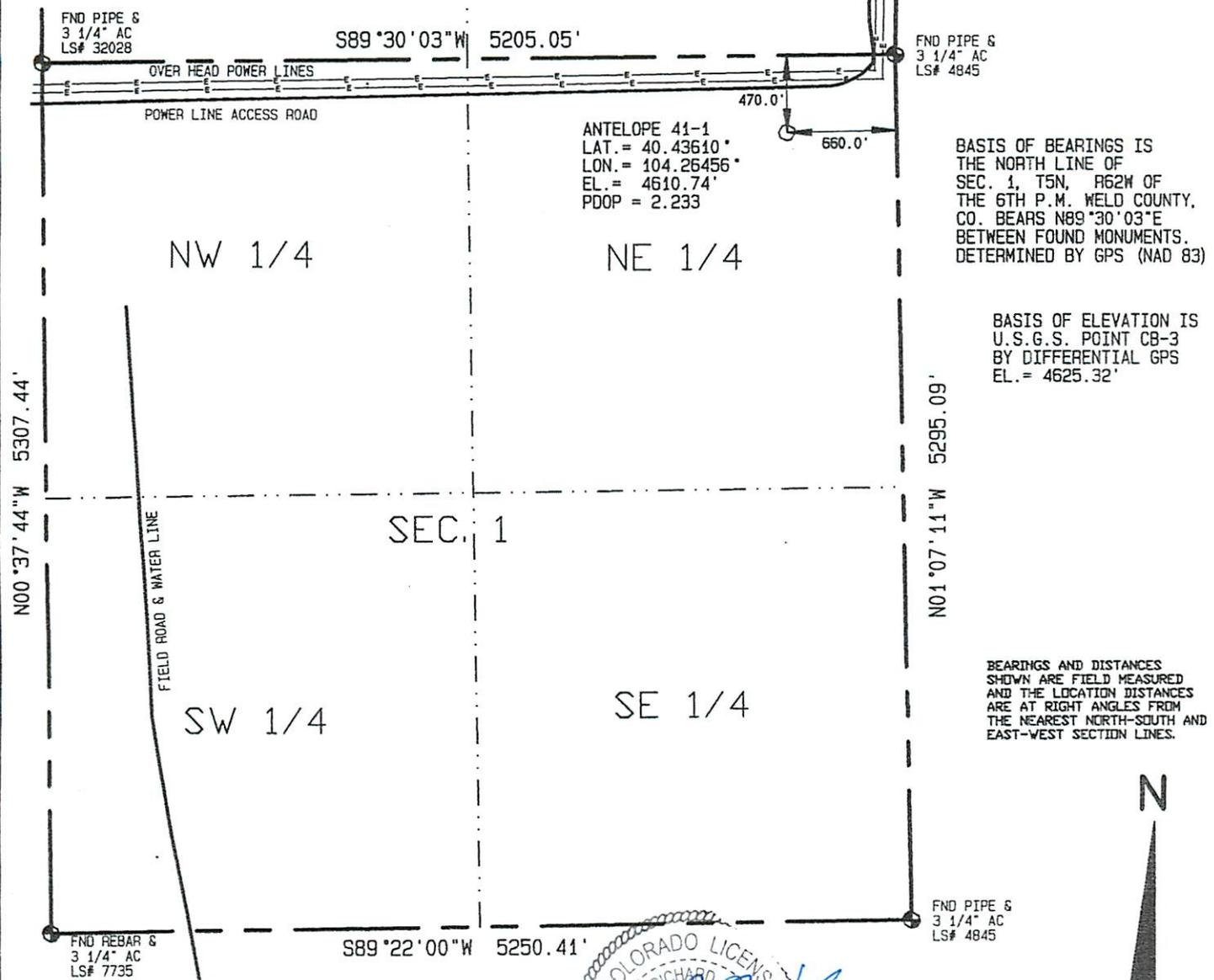
BASIS OF BEARINGS IS THE NORTH LINE OF SEC. 1, T5N, R62W OF THE 6TH P.M. WELD COUNTY, CO. BEARS N89°30'03"E BETWEEN FOUND MONUMENTS. DETERMINED BY GPS (NAD 83)
