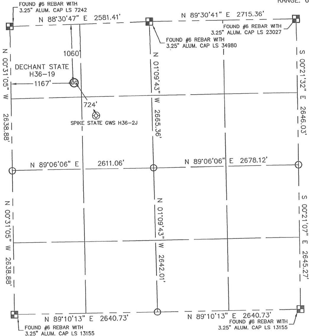
In accordance with a request from SEAN CASPER with Noble Energy Inc. Lat40°, LLC has determined the surface location of the DECHANT STATE H36-19 to be 1060' from the NORTH line and 1167' from the WEST line as measured at right angles from the section line of Section 36, Township 3 North, Range 65 West of the Sixth Principal Meridian, County of Weld, State of Colorado.
