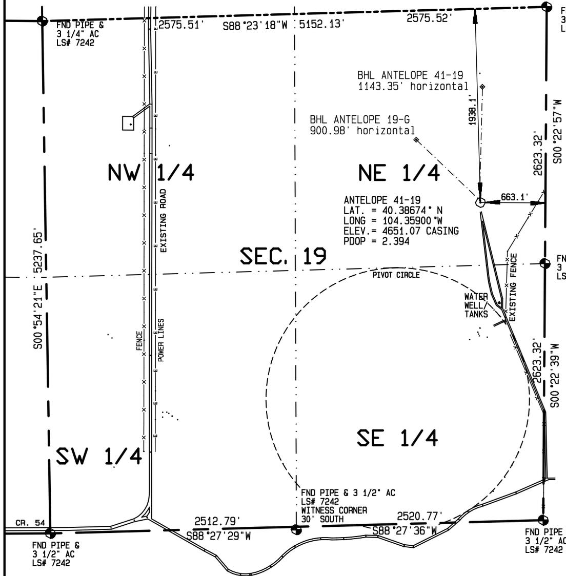
BASIS OF BEARINGS IS THE NORTH LINE SEC. 19, T5N, R62W OF THE 6TH P.M. WELD COUNTY, CO. BEARS N88°23'18"E BETWEEN SET MONUMENTS AS DETERMINED BY GPS (NAD 83)
