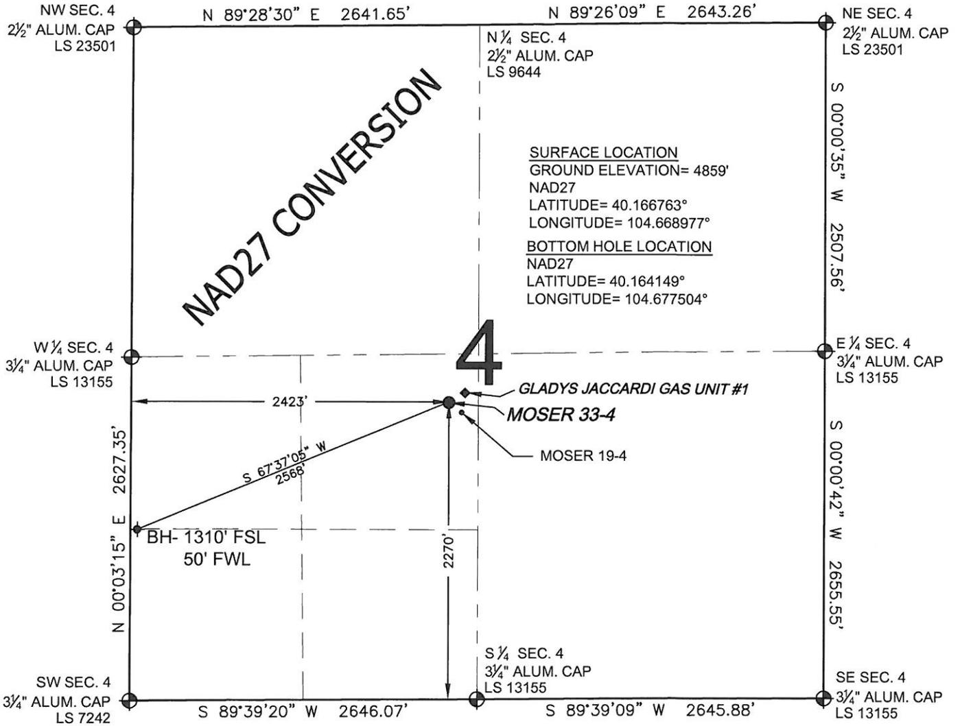
WELL **MOSER 33-4** TO BE LOCATED 2270' FSL AND 2423' FWL, SECTION 4, T2N, R65W OF THE 6th P.M.
