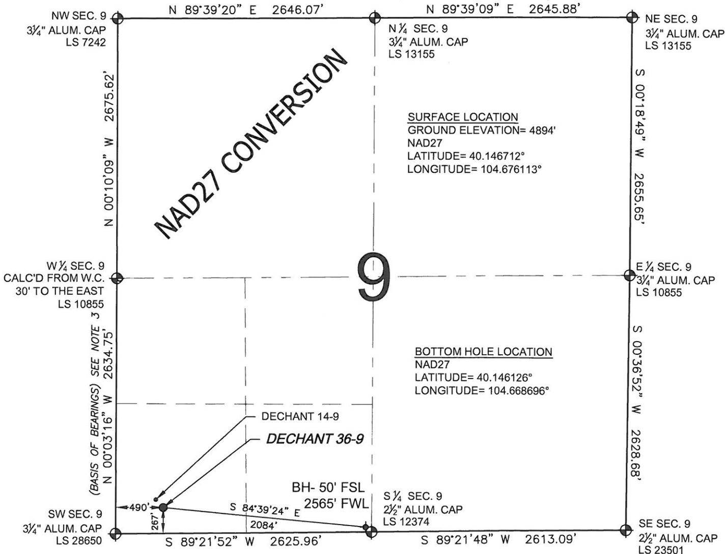
WELL **DECHANT 36-9** TO BE LOCATED 267' FSL AND 490' FWL, SECTION 9, T2N, R65W OF THE 6th P.M.
