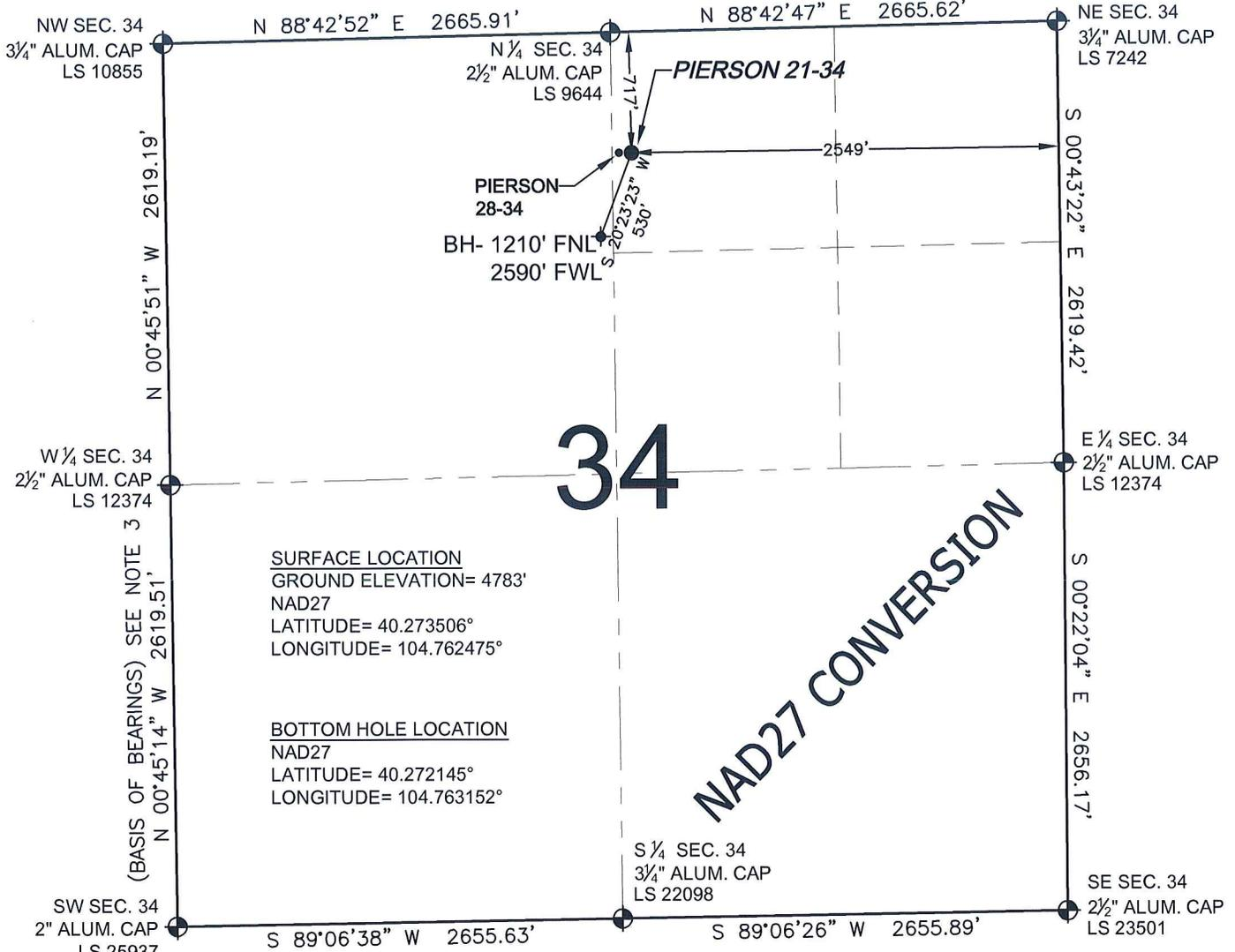
WELL **PIERSON 21-34** TO BE LOCATED 717' FNL AND 2549' FEL, SECTION 34, T4N, R66W OF THE 6TH P.M.
