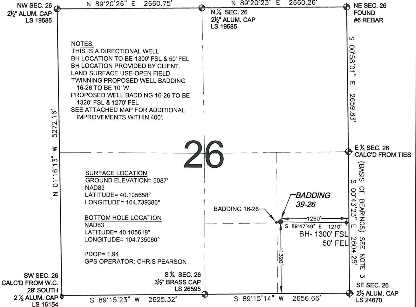
WELL **BADDING 39-26** TO BE LOCATED 1320' FSL AND 1260' FEL, SECTION 26, T2N, R66W OF THE 6th P.M.
