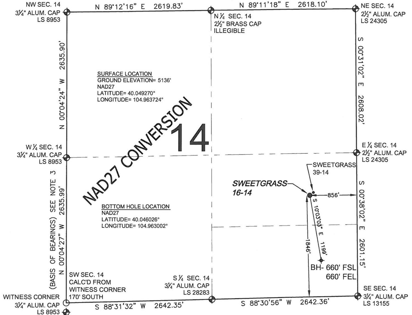
WELL **SWEETGRASS 16-14** TO BE LOCATED 1846' FSL AND 856' FEL, SECTION 14, T1N, R68W OF THE 6th P.M.
