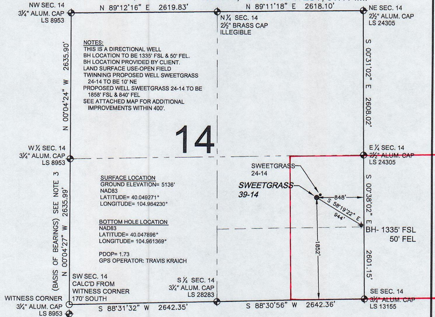
WELL **SWEETGRASS 39-14** TO BE LOCATED 1852' FSL AND 848' FEL, SECTION 14, T1N, R68W OF THE 6TH P.M.
