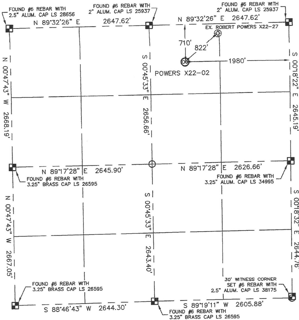
In accordance with a request from Mike Rodine with Noble Energy Inc. Lat40°, LLC has determined the surface location of the POWERS X22-02 to be 710' from the NORTH line and 1980' from the EAST line as measured at right angles from the section line of Section 22, Township 2 North, Range 65 West of the Sixth Principal Meridian, County of Weld, State of Colorado.
