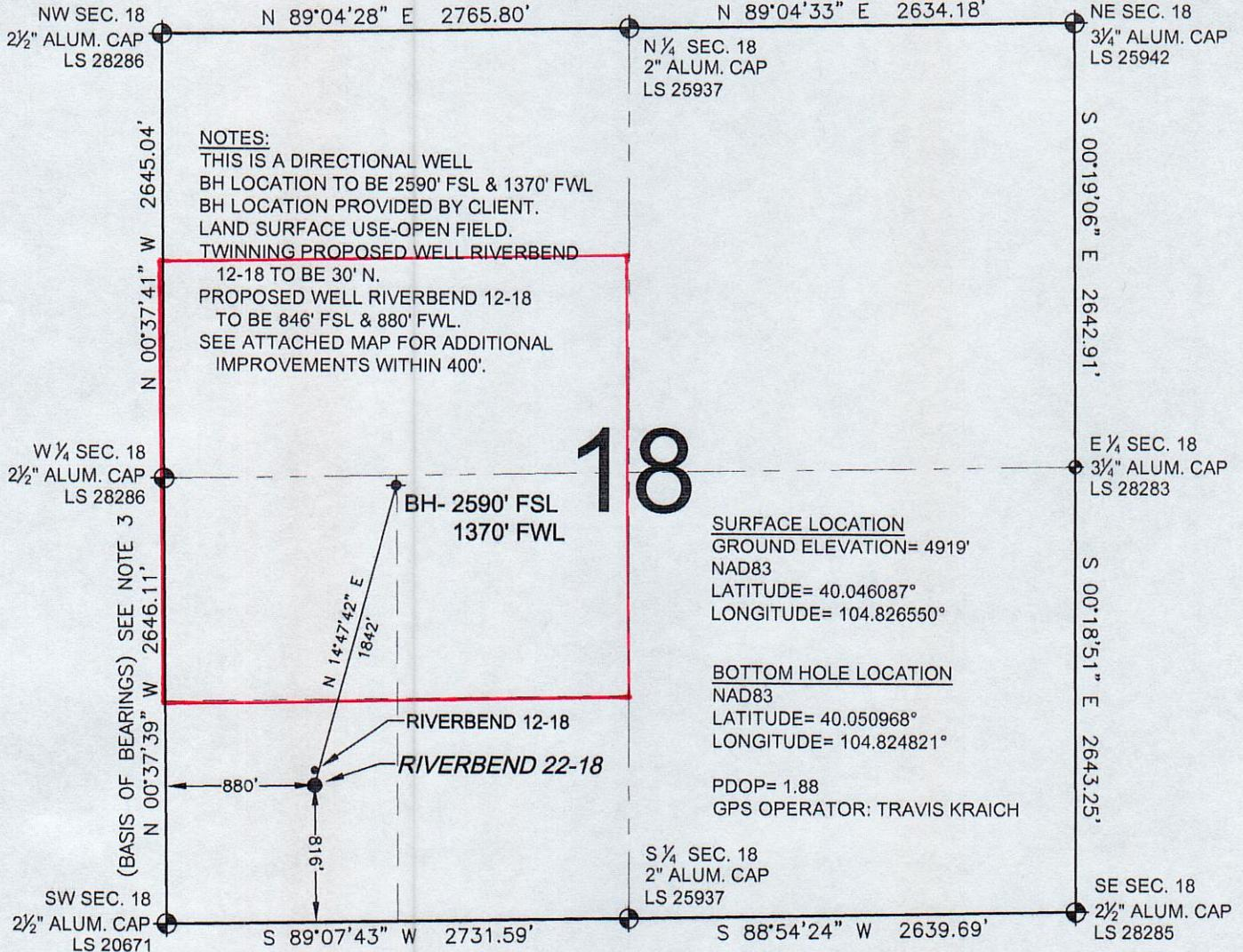
WELL RIVERBEND 22-18 TO BE LOCATED 816' FSL AND 880' FWL, SECTION 18, T1N, R66W OF THE 6th P.M.
