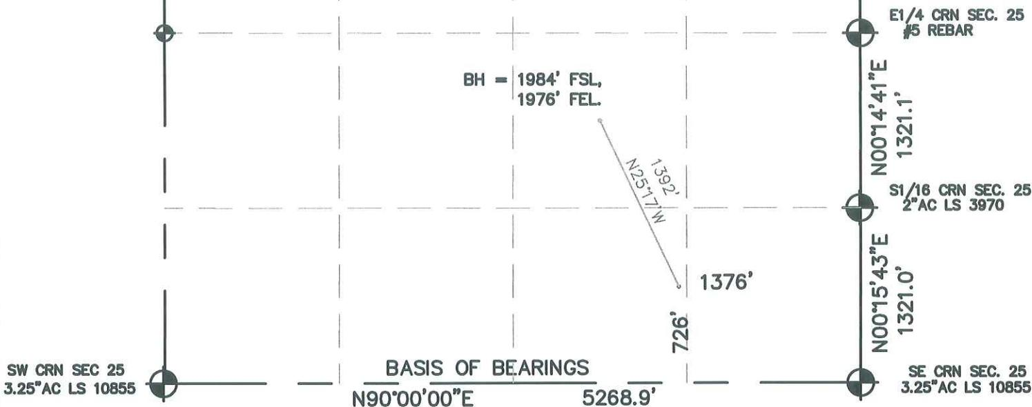
I HEREBY STATE TO PETROLEUM DEVELOPMENT CORP. THAT THIS WELL LOCATION CERTIFICATE FOR THE WELL COORS ENERGY 33-25D IS LOCATED 726' FSL & 1376' FEL, SEC. 25, T3N, R64W, 6PM.
