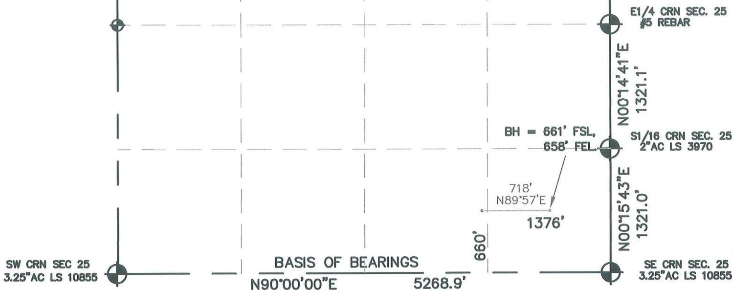
I HEREBY STATE TO PETROLEUM DEVELOPMENT CORP. THAT THIS WELL LOCATION CERTIFICATE FOR THE WELL COORS ENERGY 44-25D IS LOCATED 660' FSL & 1376' FEL, SEC. 25, T3N, R64W, 6PM.
