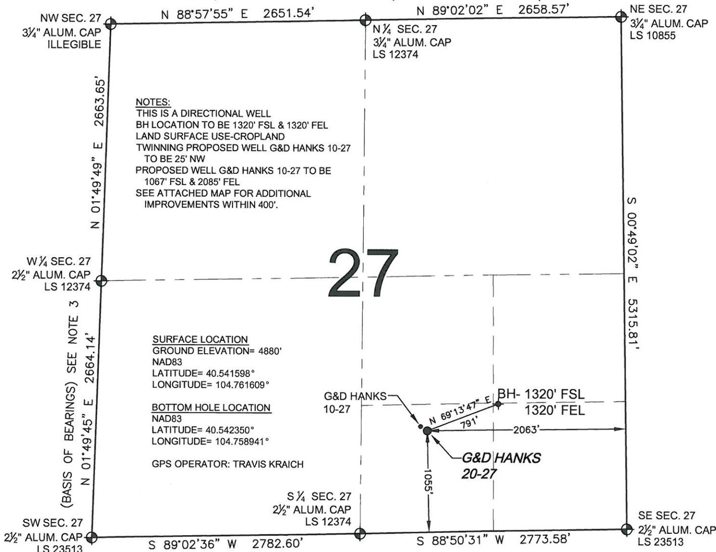
WELL **G&D HANKS 20-27** TO BE LOCATED 1055' FSL AND 2063' FEL, SECTION 27, T7N, R66W OF THE 6th P.M.
