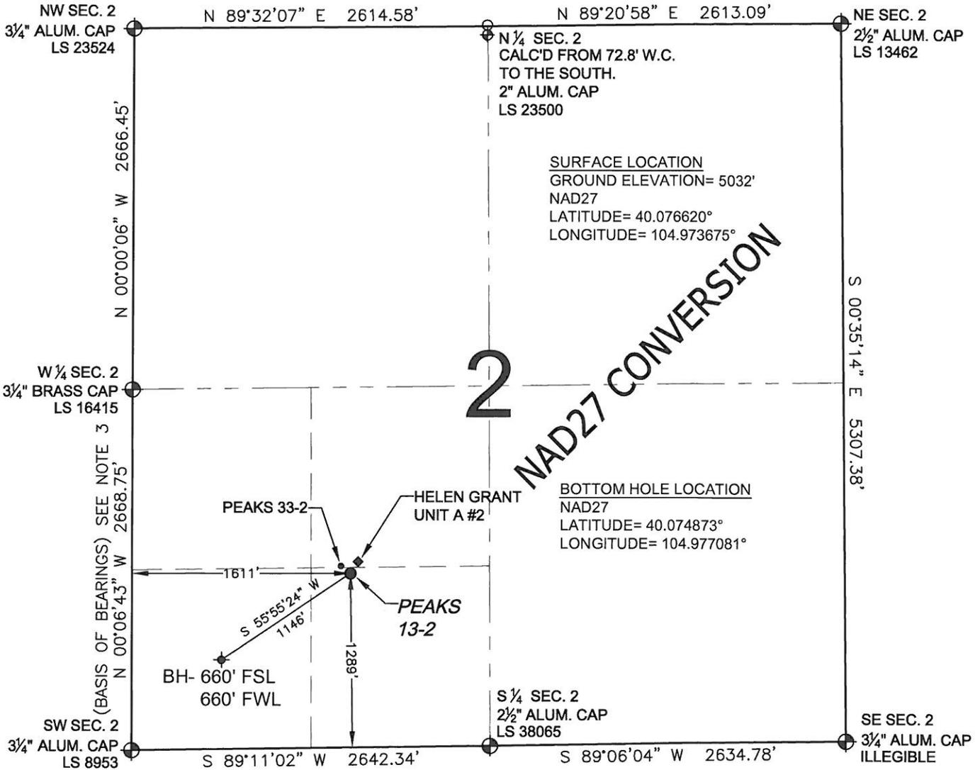
WELL **PEAKS 13-2** TO BE LOCATED 1289' FSL AND 1611' FWL, SECTION 2, T1N, R68W OF THE 6th P.M.
