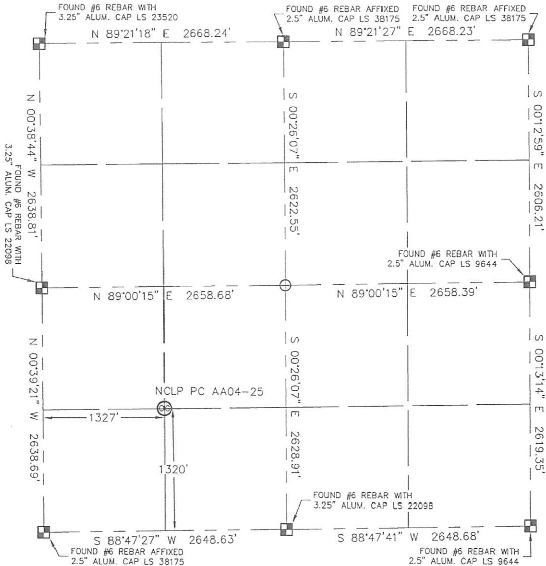
In accordance with a request from ROBBIE MILLER with Noble Energy Inc., Lat40°, LLC has determined the surface location of the NCLP PC AA04-25 to be 1320' from the SOUTH line and 1327' from the WEST line as measured at right angles from the section line of Section 4, Township 6 North, Range 63 West of the Sixth Principal Meridian, County of Weld, State of Colorado.
