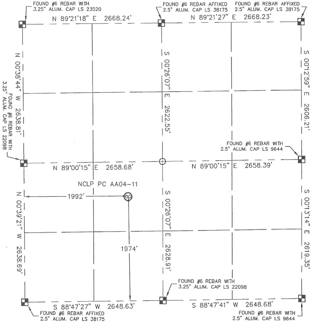
In accordance with a request from ROBBIE MILLER with Noble Energy Inc., Lat40°, LLC has determined the surface location of the NCLP PC AA04-11 to be 1974' from the SOUTH line and 1992' from the WEST line as measured at right angles from the section line of Section 4, Township 6 North, Range 63 West of the Sixth Principal Meridian, County of Weld, State of Colorado.
