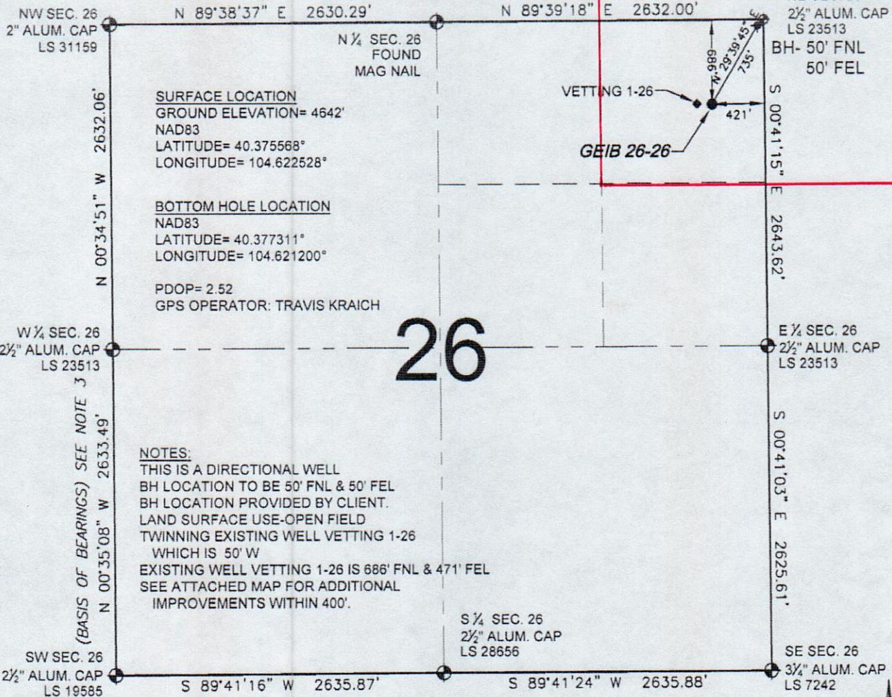
WELL **GEIB 26-26** TO BE LOCATED 686' FNL AND 421' FEL, SECTION 26, T5N, R65W OF THE 6th P.M.
