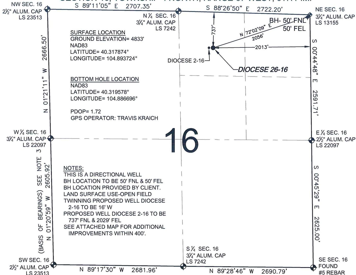
WELL **DIOCESE 26-16** TO BE LOCATED 737' FNL AND 2013' FEL, SECTION 16, T4N, R67W OF THE 6th P.M.
