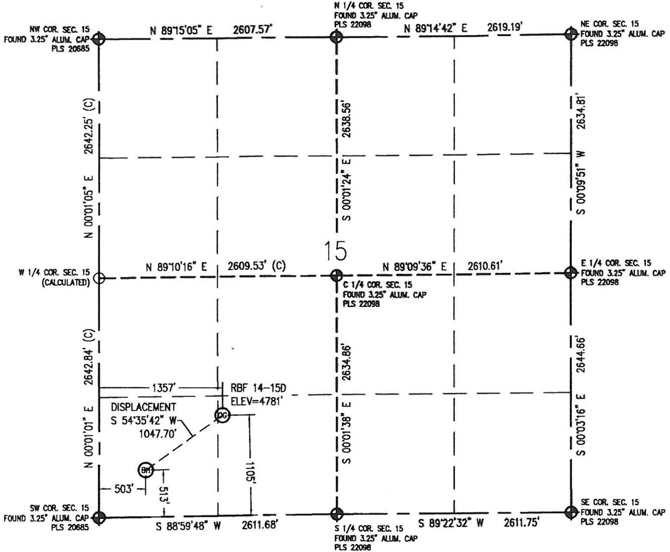
IN ACCORDANCE WITH A REQUEST FROM CRAIG RASMUSON - SYNERGY RESOURCES CORP., BASELINE ENGINEERING CORP. HAS DETERMINED THE LOCATION OF THE RBF 14-15D TO BE 1105' FSL AND 1357' FWL, AS MEASURED AT NINETY (90) DEGREES FROM THE SECTION LINE OF SECTION 15, TOWNSHIP 6 NORTH, RANGE 67 WEST AND THE BOTTOM HOLE LOCATION TO BE 513' FSL AND 503' FWL OF SECTION 15, TOWNSHIP 6 NORTH, RANGE 67 WEST, 6TH PRINCIPAL MERIDIAN, WELD COUNTY, COLORADO.
