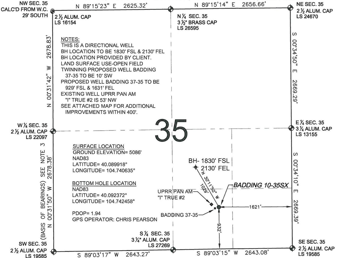
WELL **BADDING 10-35SX** TO BE LOCATED 932' FSL AND 1621' FEL, SECTION 35, T2N, R66W OF THE 6th P.M.
