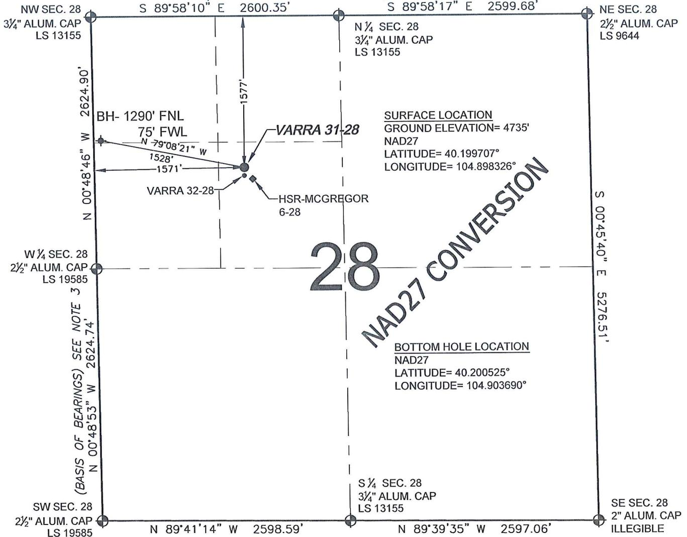
WELL VARRA 31-28 TO BE LOCATED 1577' FNL AND 1571' FWL, SECTION 28, T3N, R67W OF THE 6th P.M.
