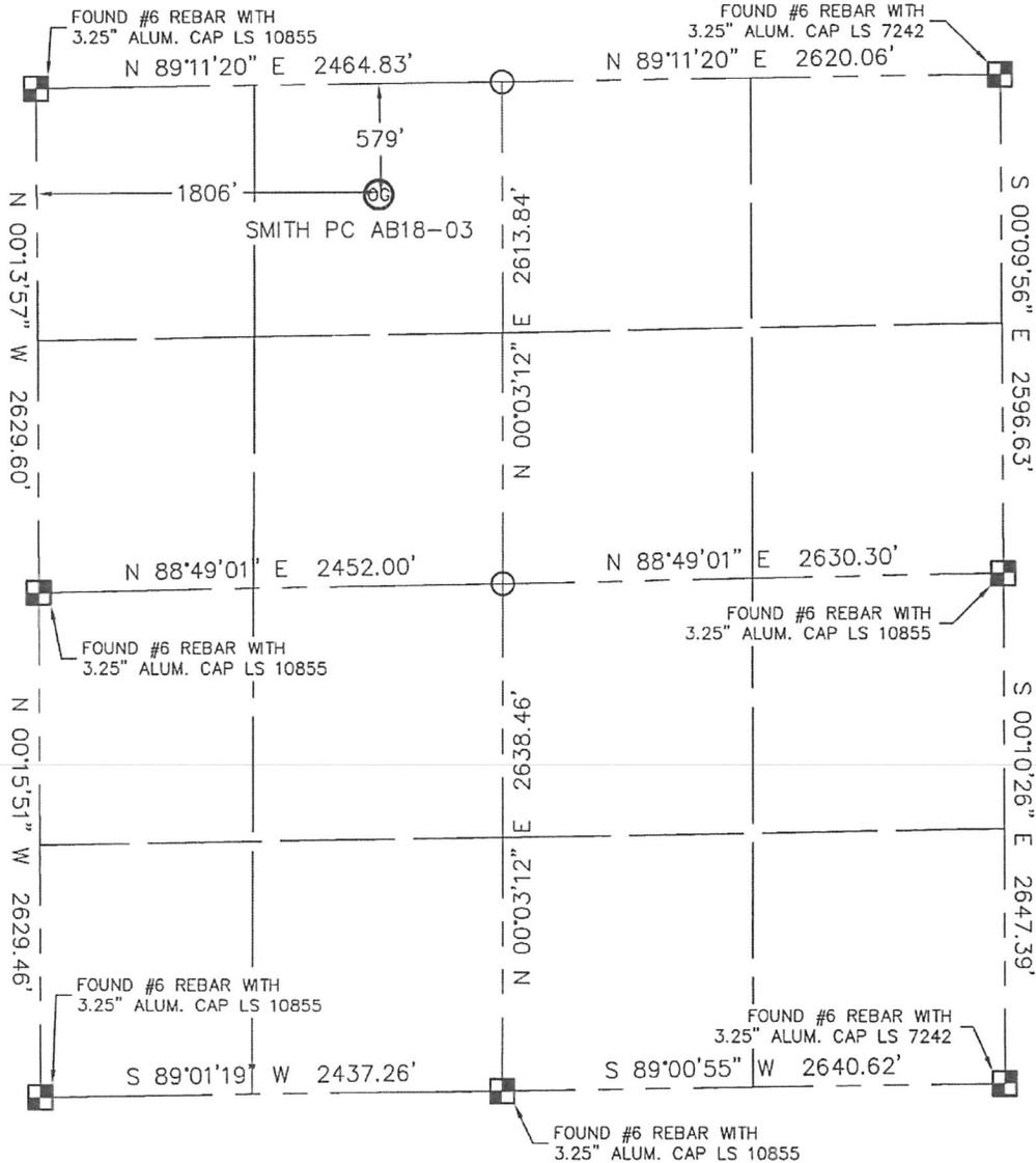
In accordance with a request from RYAN ANTONIO with Noble Energy Inc., Lat40°, LLC has determined the surface location of the SMITH PC AB18-03 to be 579' from the NORTH line and 1806' from the WEST line as measured at right angles from the section line of Section 18, Township 7 North, Range 64 West of the Sixth Principal Meridian, County of Weld, State of Colorado.
