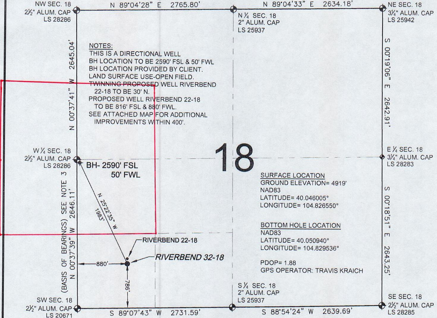
WELL RIVERBEND 32-18 TO BE LOCATED 786' FSL AND 880' FWL, SECTION 18, T1N, R66W OF THE 6th P.M.
