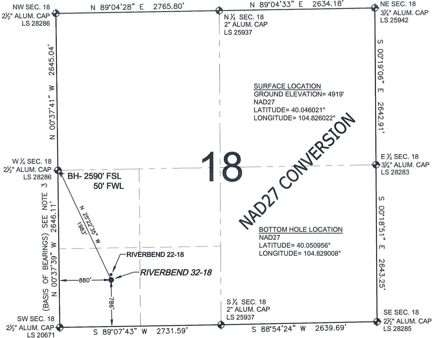
**WELL RIVERBEND 32-18 TO BE LOCATED 786' FSL AND 880' FWL, SECTION 18, T1N, R66W OF THE 6th P.M.**
