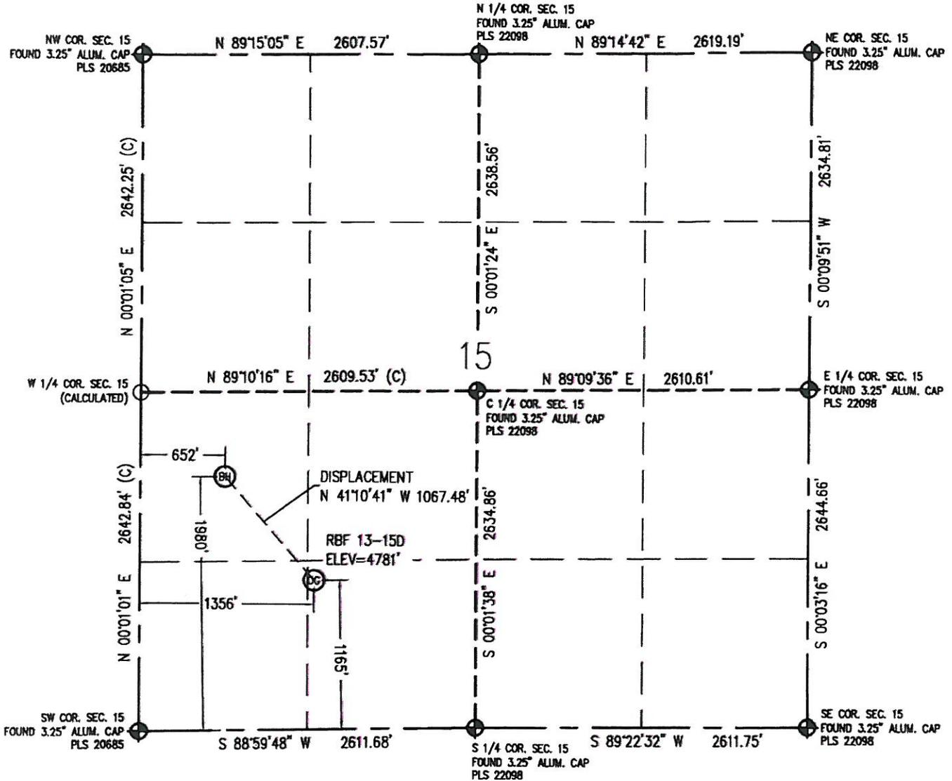
IN ACCORDANCE WITH A REQUEST FROM CRAIG RASMUSON - SYNERGY RESOURCES CORP., BASELINE ENGINEERING CORP. HAS DETERMINED THE LOCATION OF THE RBF 13-150 TO BE 1165' FSL AND 1356' FWL, AS MEASURED AT NINETY (90) DEGREES FROM THE SECTION LINE OF SECTION 15, TOWNSHIP 6 NORTH, RANGE 67 WEST AND THE BOTTOM HOLE LOCATION TO BE 1986' FSL AND 652' FWL OF SECTION 15, TOWNSHIP 6 NORTH, RANGE 67 WEST, 6TH PRINCIPAL MERIDIAN, WELD COUNTY, COLORADO.
