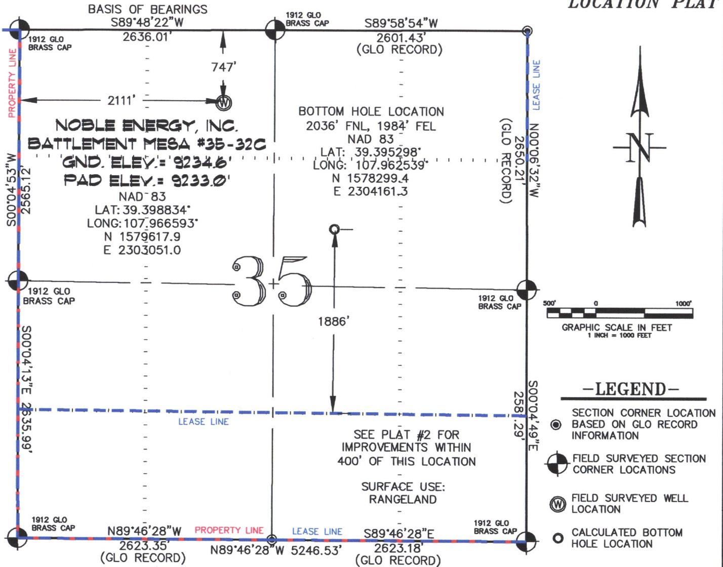
**THIS WELL LOCATION PLAT WAS PREPARED FOR NOBLE ENERGY INC. TO LOCATE THE BATTLEMENT MESA #35-32C WELL, 747 FEET FROM THE NORTH LINE AND 2111 FEET FROM THE WEST LINE IN THE NE1/4 NW1/4 OF SECTION 35, T. 7 S., R. 95 W. OF THE 6TH P.M. GARFIELD COUNTY, COLORADO.**
