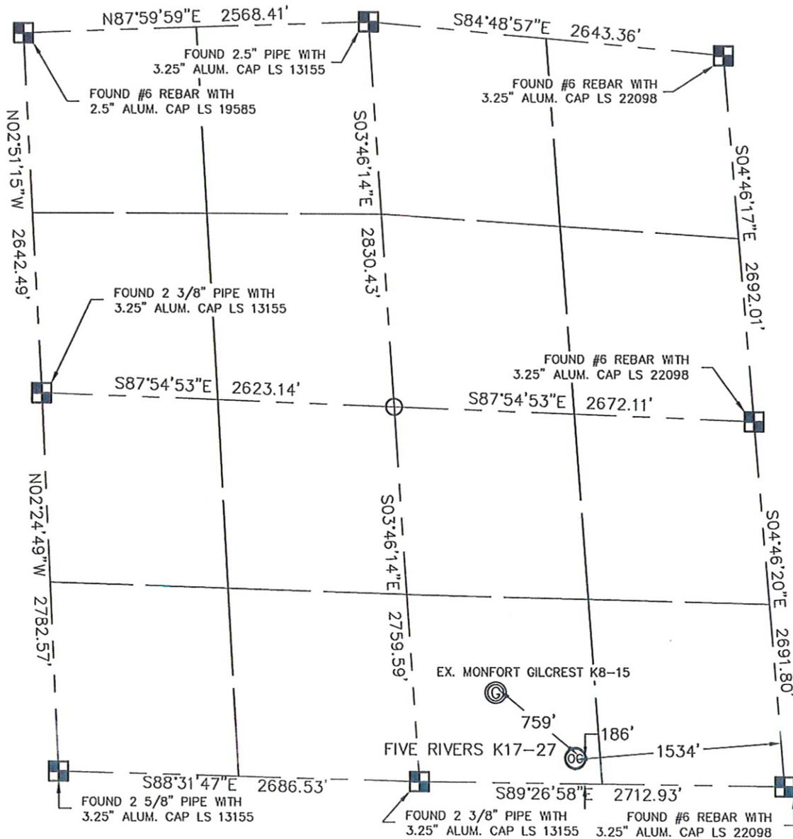
In accordance with a request from JOE MARTIN with Noble Energy Inc., King Surveyors Inc. has determined the surface location of the FIVE RIVERS K17-27 to be 186' from the SOUTH line and 1534' from the EAST line as measured at right angles from the section line of Section 8, Township 4 North, Range 66 West of the Sixth Principal Meridian, County of Weld, State of Colorado.
