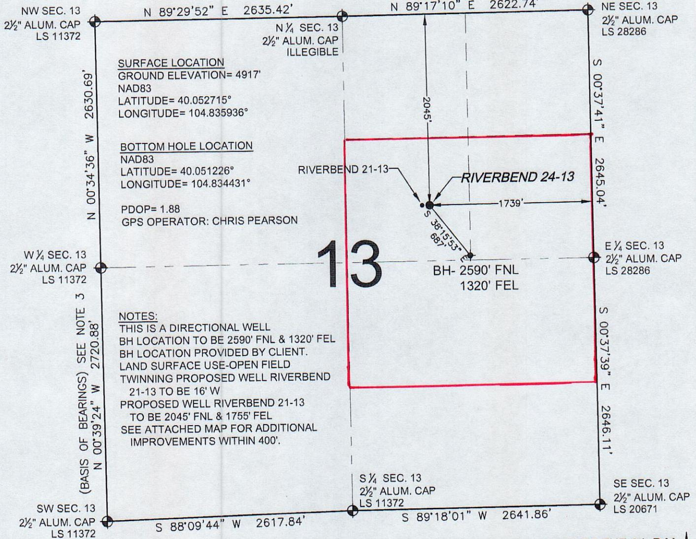
WELL **RIVERBEND 24-13** TO BE LOCATED 2045' FNL AND 1739' FEL, SECTION 13, T1N, R67W OF THE 6th P.M.
