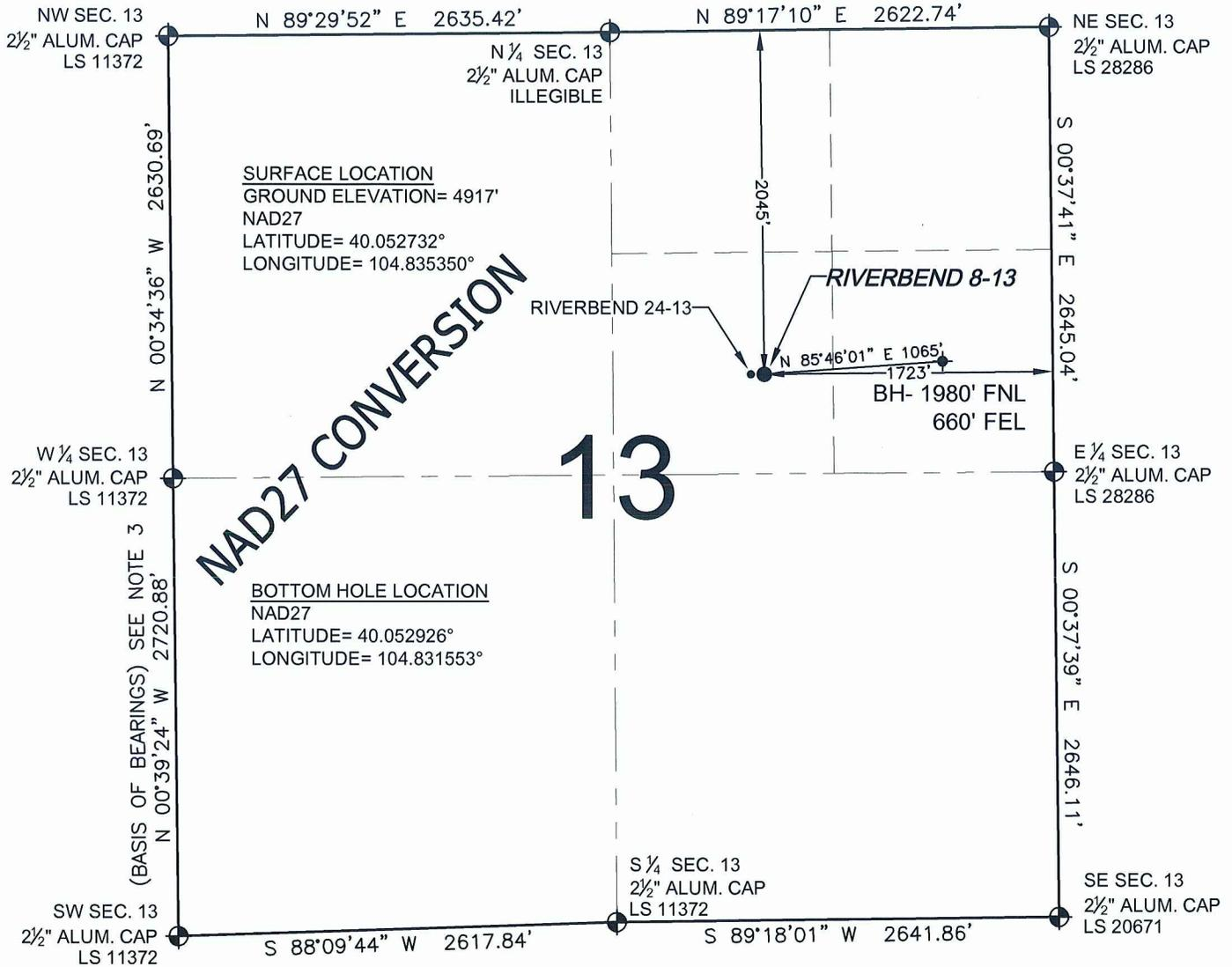
WELL **RIVERBEND 8-13** TO BE LOCATED 2045' FNL AND 1723' FEL, SECTION 13, T1N, R67W OF THE 6th P.M.
