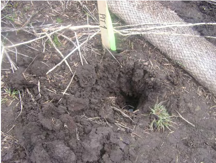
Photo 5: Pit 4, note water in pit ponding on top of impermeable liner
