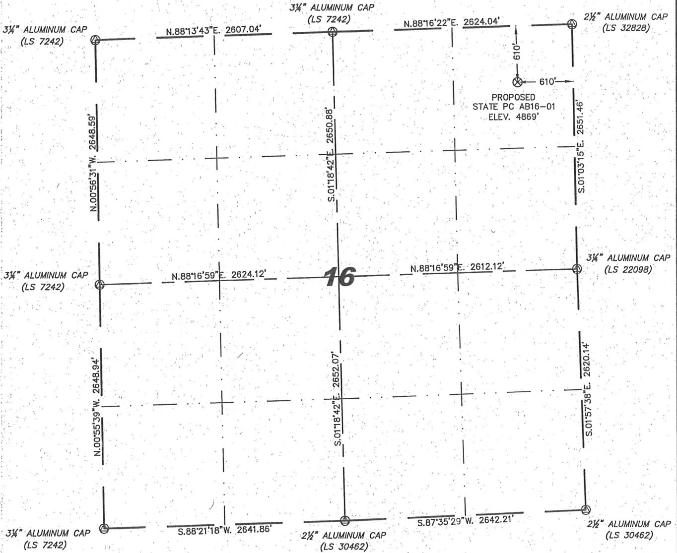
IN ACCORDANCE WITH A REQUEST FROM ERIK VAN DECAR - NOBLE ENERGY INC, STEIL SURVEYING SERVICES, LLC HAS DETERMINED THE LOCATION OF THE STATE PC AB16-01 WELL TO BE 610' FNL, 610' FEL, AS MEASURED AT NINETY (90) DEGREES FROM THE SECTION LINES, SECTION 16, TOWNSHIP 7 NORTH, RANGE 64 WEST, 6TH PRINCIPLE MERIDIAN, WELD COUNTY, COLORADO.
