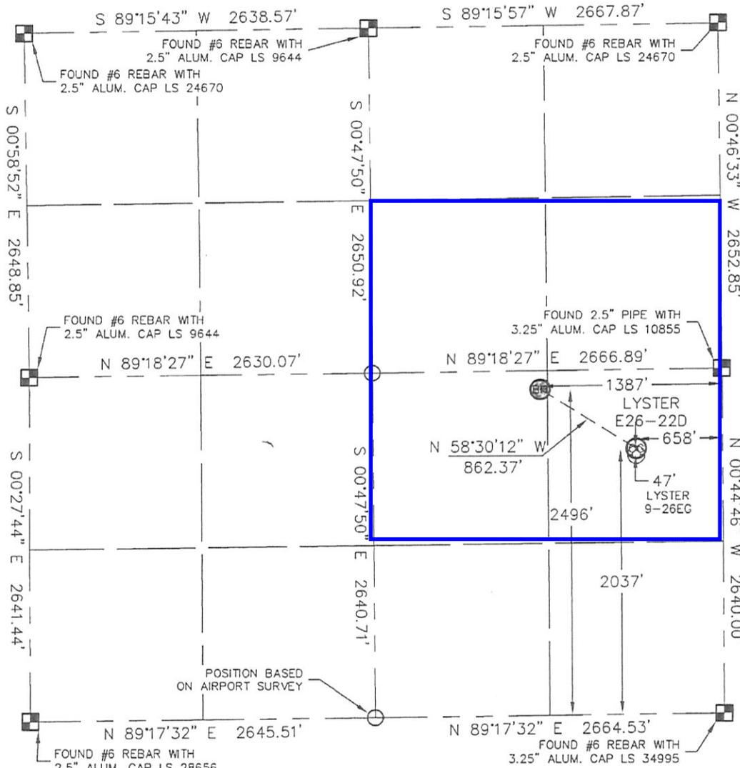
In accordance with a request from BEAU FRITZ with Noble Energy Inc. Lat40°, LLC has determined the surface location of the LYSTER E26-22D to be 2037' from the SOUTH line and 658' from the EAST line and the bottom hole to be 2496' from the SOUTH line and 1387' from the EAST line as measured at right angles from the section line of Section 26, Township 6 North, Range 65 West of the Sixth Principal Meridian, County of Weld, State of Colorado.
