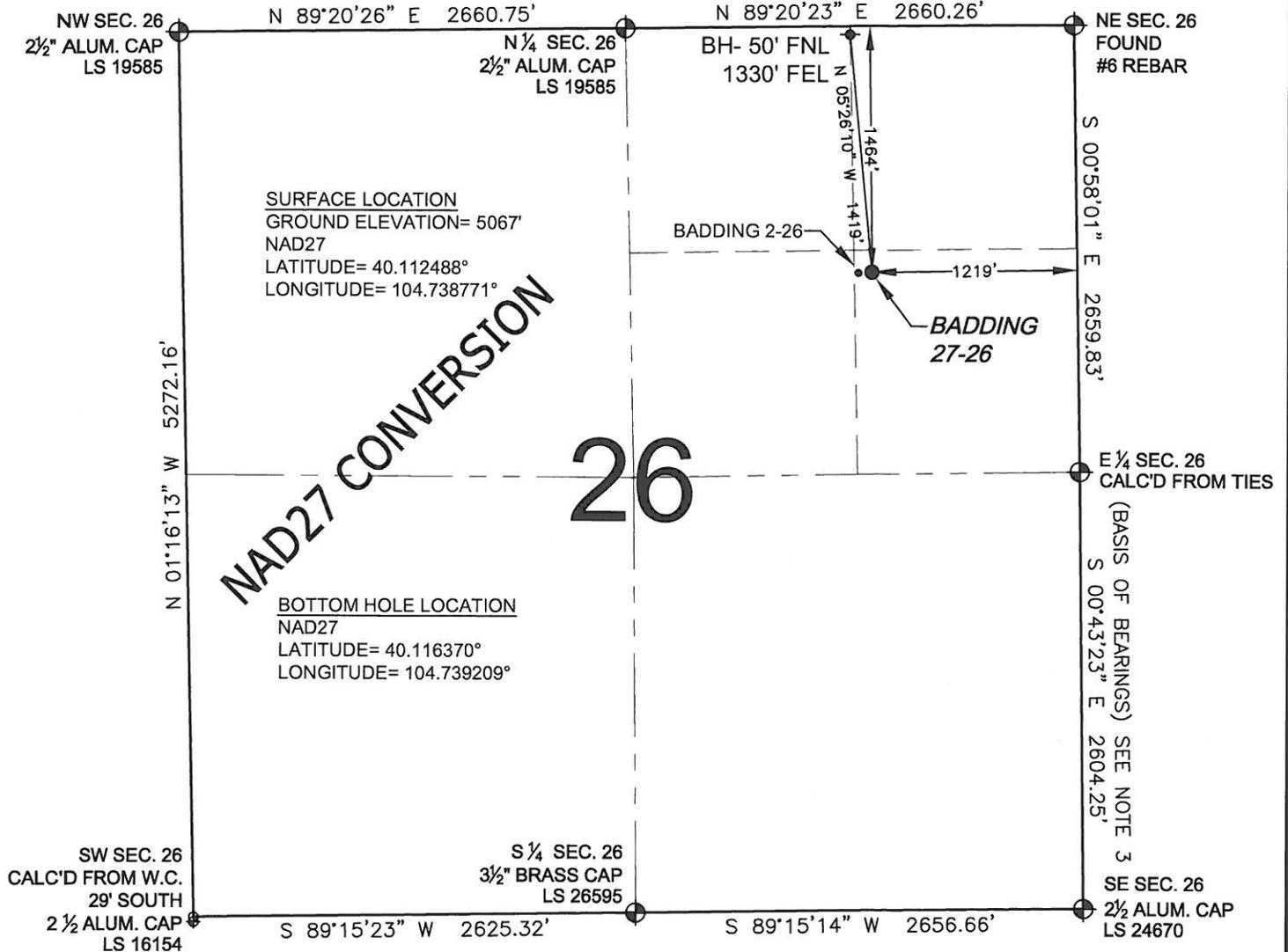
WELL **BADDING 27-26** TO BE LOCATED 1464' FNL AND 1219' FEL, SECTION 26, T2N, R66W OF THE 6th P.M.
