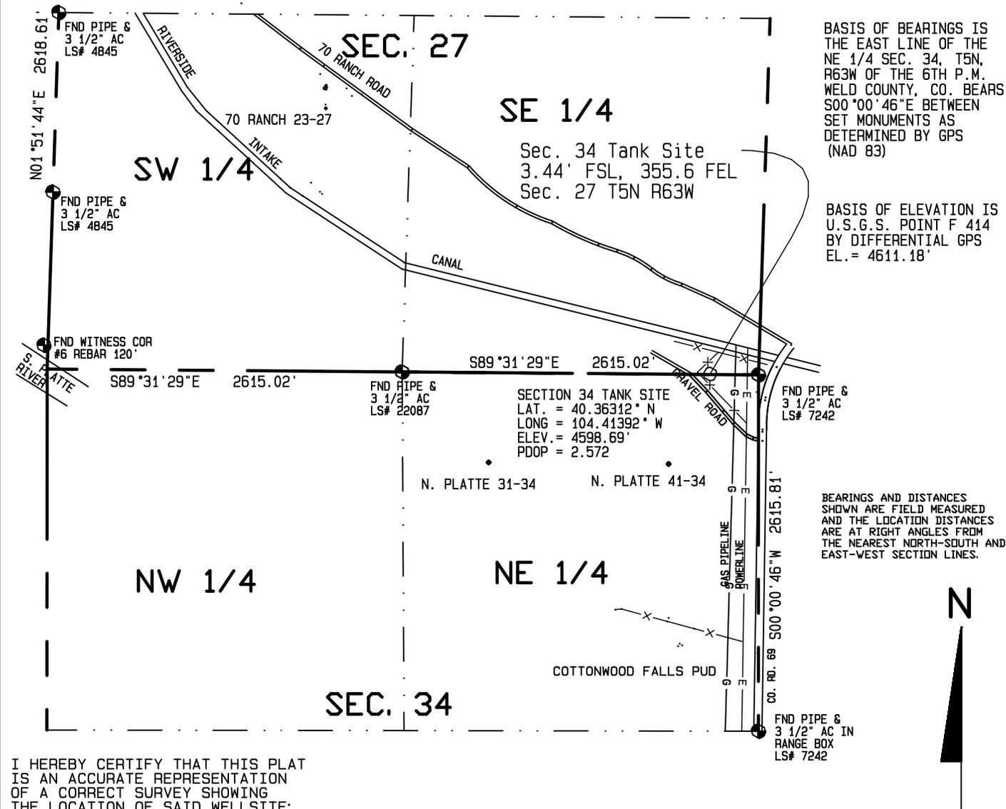
BASIS OF BEARINGS IS THE EAST LINE OF THE NE 1/4 SEC. 34, T5N, R63W OF THE 6TH P.M. WELD COUNTY, CO. BEARS S00°00'46\"E BETWEEN SET MONUMENTS AS DETERMINED BY GPS (NAD 83)
