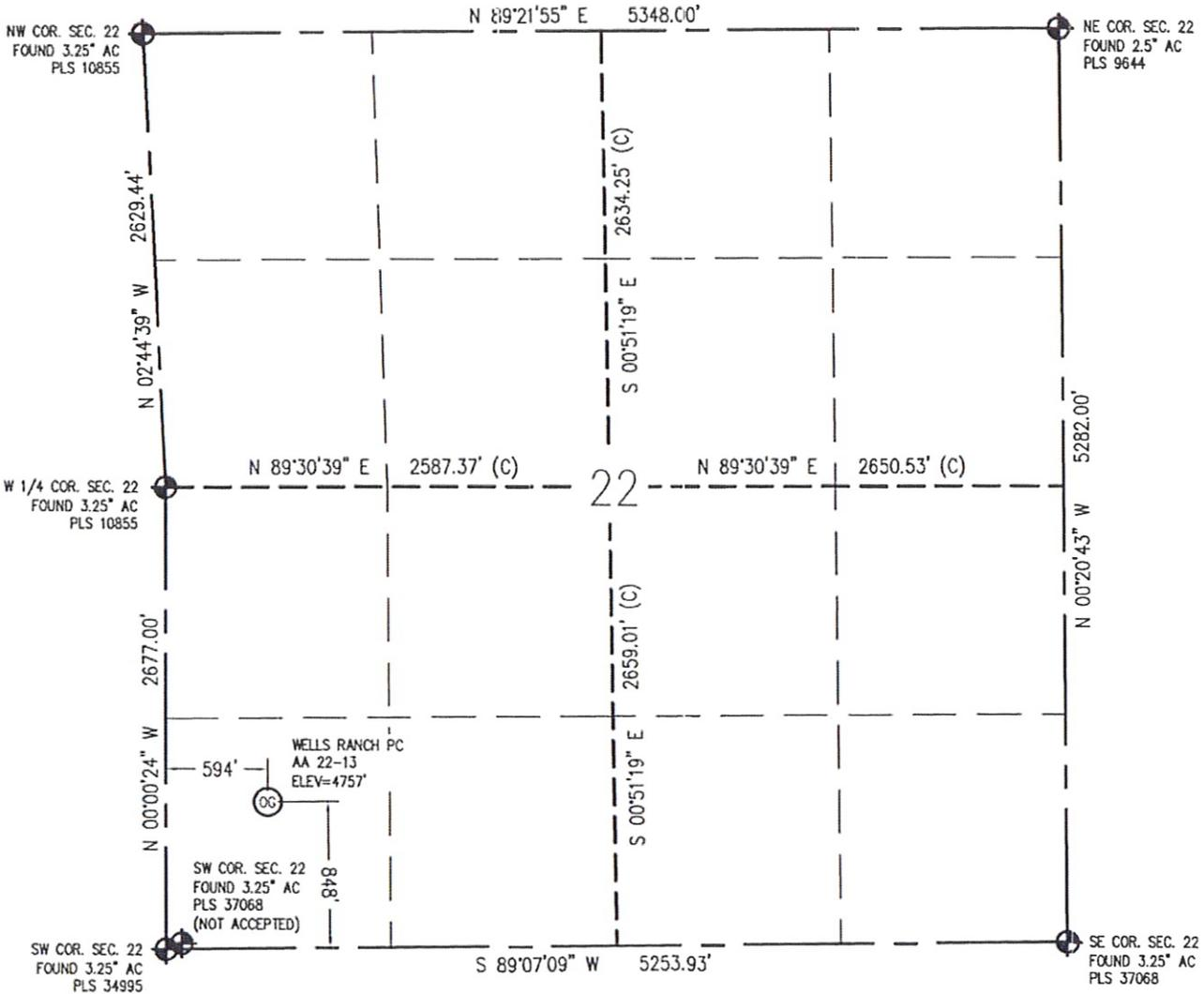
IN ACCORDANCE WITH A REQUEST FROM SEAN CASPER - NOBLE ENERGY INC., BASELINE ENGINEERING CORP. HAS DETERMINED THE LOCATION OF THE WELLS RANCH PC AA 22-13 TO BE 594' FWL AND 848' FSL, AS MEASURED AT NINETY (90) DEGREES FROM THE SECTION LINE OF SECTION 22, TOWNSHIP 6 NORTH, RANGE 63 WEST, 6TH PRINCIPAL MERIDIAN, WELD COUNTY, COLORADO.
