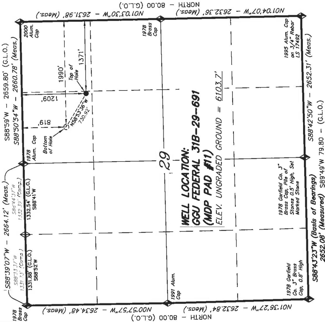
WELL LOCATION, GGU FEDERAL 31B-29-691 (MDP PAD #11), LOCATED AS SHOWN IN THE NW 1/4 NE 1/4 OF SECTION 29, T6S, R91W, 6th P.M. GARFIELD COUNTY, COLORADO.
