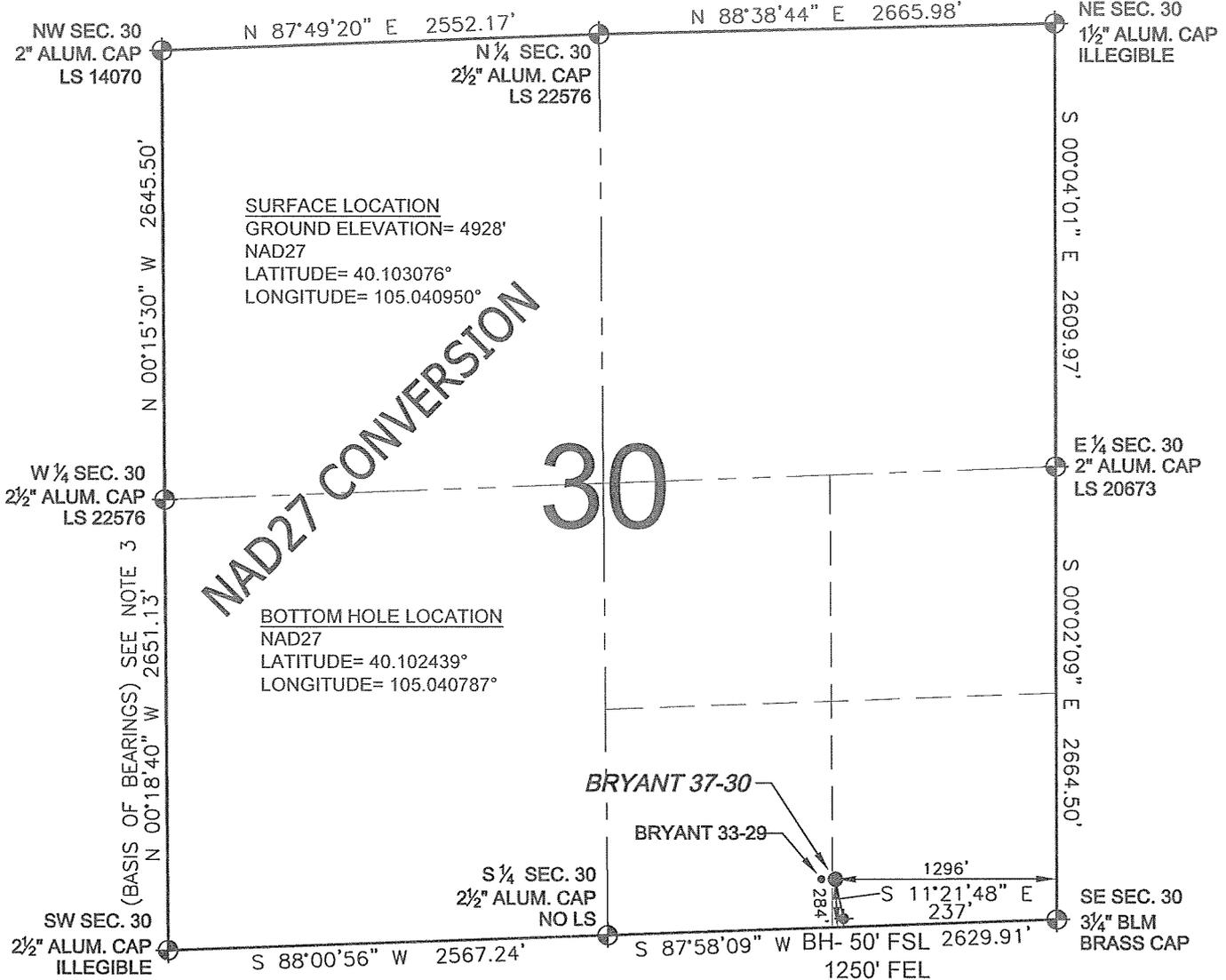
WELL **BRYANT 37-30** TO BE LOCATED 284' FSL AND 1296' FEL, SECTION 30, T2N, R68W OF THE 6th P.M.
