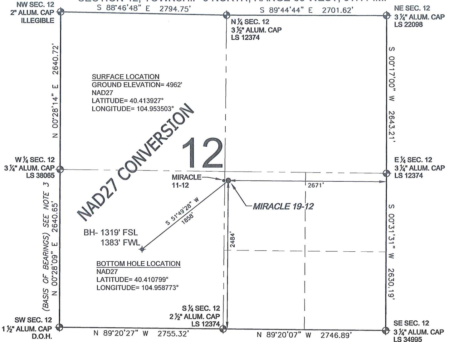
WELL **MIRACLE 19-12** TO BE LOCATED 2484' FSL AND 2671' FEL, SECTION 12, T5N, R68W OF THE 6th P.M.
