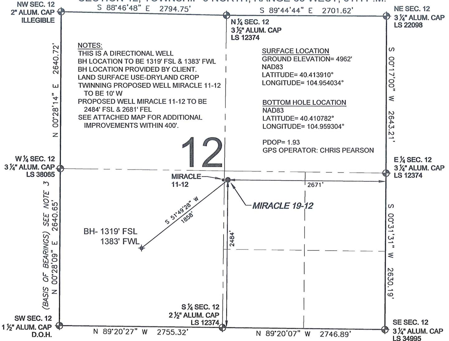
WELL **MIRACLE 19-12** TO BE LOCATED 2484' FSL AND 2671' FEL, SECTION 12, T5N, R68W OF THE 6th P.M.
