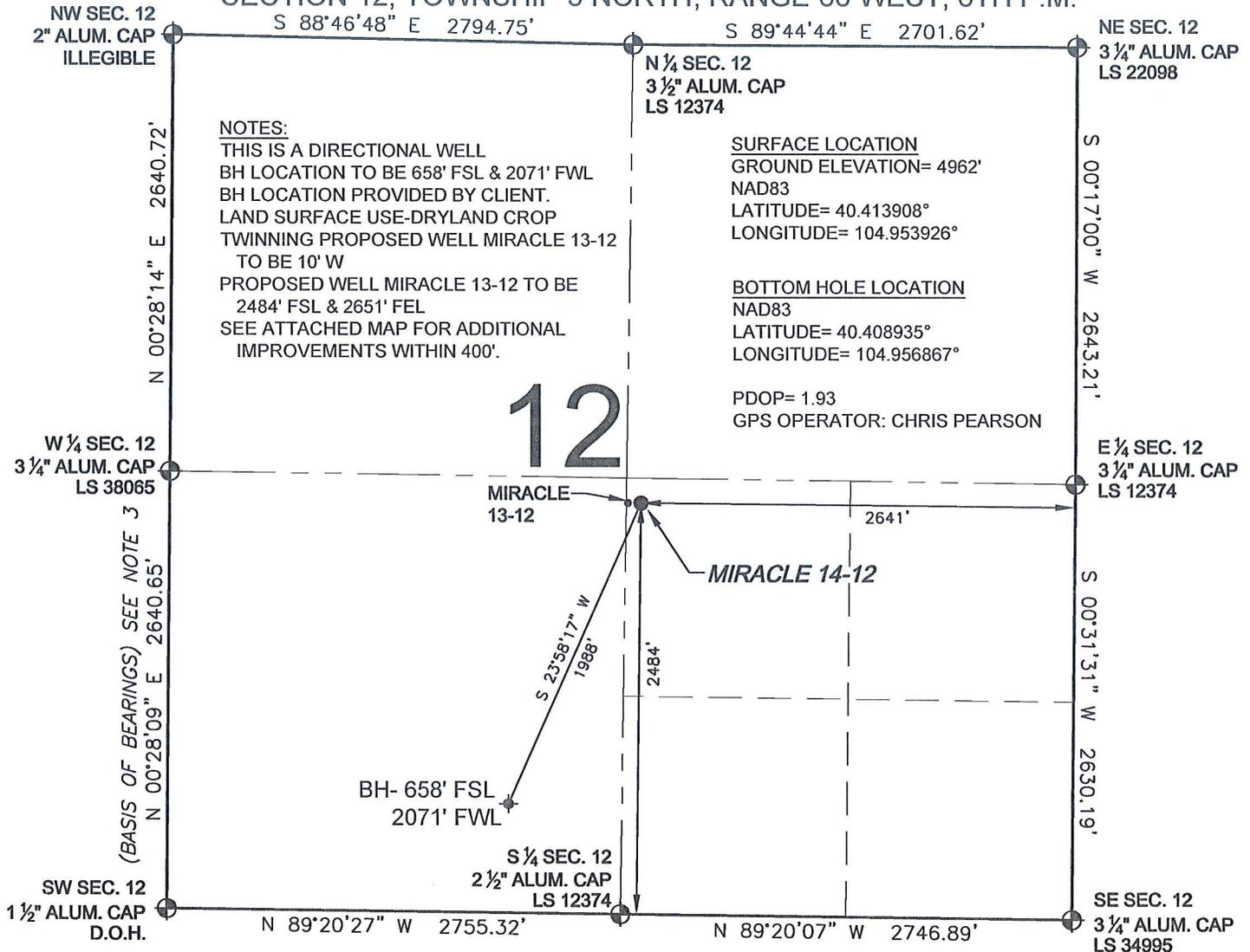
WELL **MIRACLE 14-12** TO BE LOCATED 2484' FSL AND 2641' FEL, SECTION 12, T5N, R68W OF THE 6th P.M.
