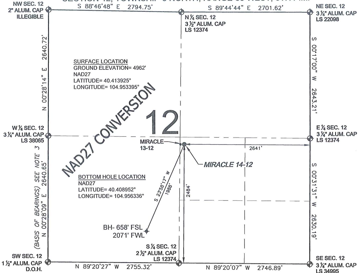
WELL MIRACLE 14-12 TO BE LOCATED 2484' FSL AND 2641' FEL, SECTION 12, T5N, R68W OF THE 6th P.M.
