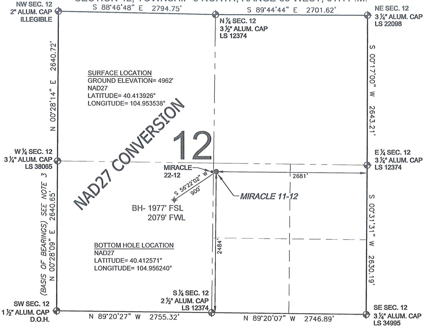
WELL **MIRACLE 11-12** TO BE LOCATED 2484' FSL AND 2681' FEL, SECTION 12, T5N, R68W OF THE 6th P.M.
