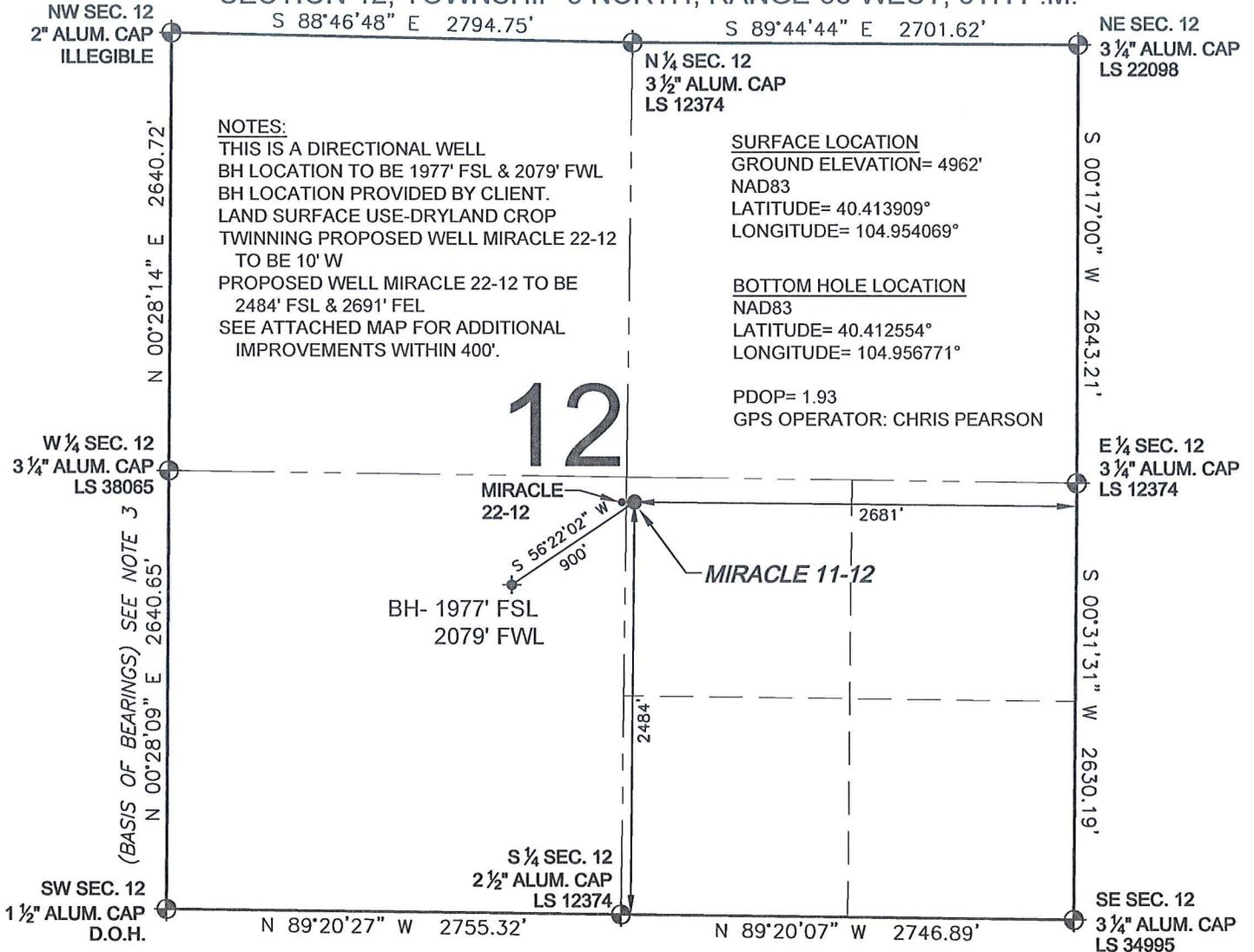
WELL **MIRACLE 11-12** TO BE LOCATED 2484' FSL AND 2681' FEL, SECTION 12, T5N, R68W OF THE 6th P.M.
