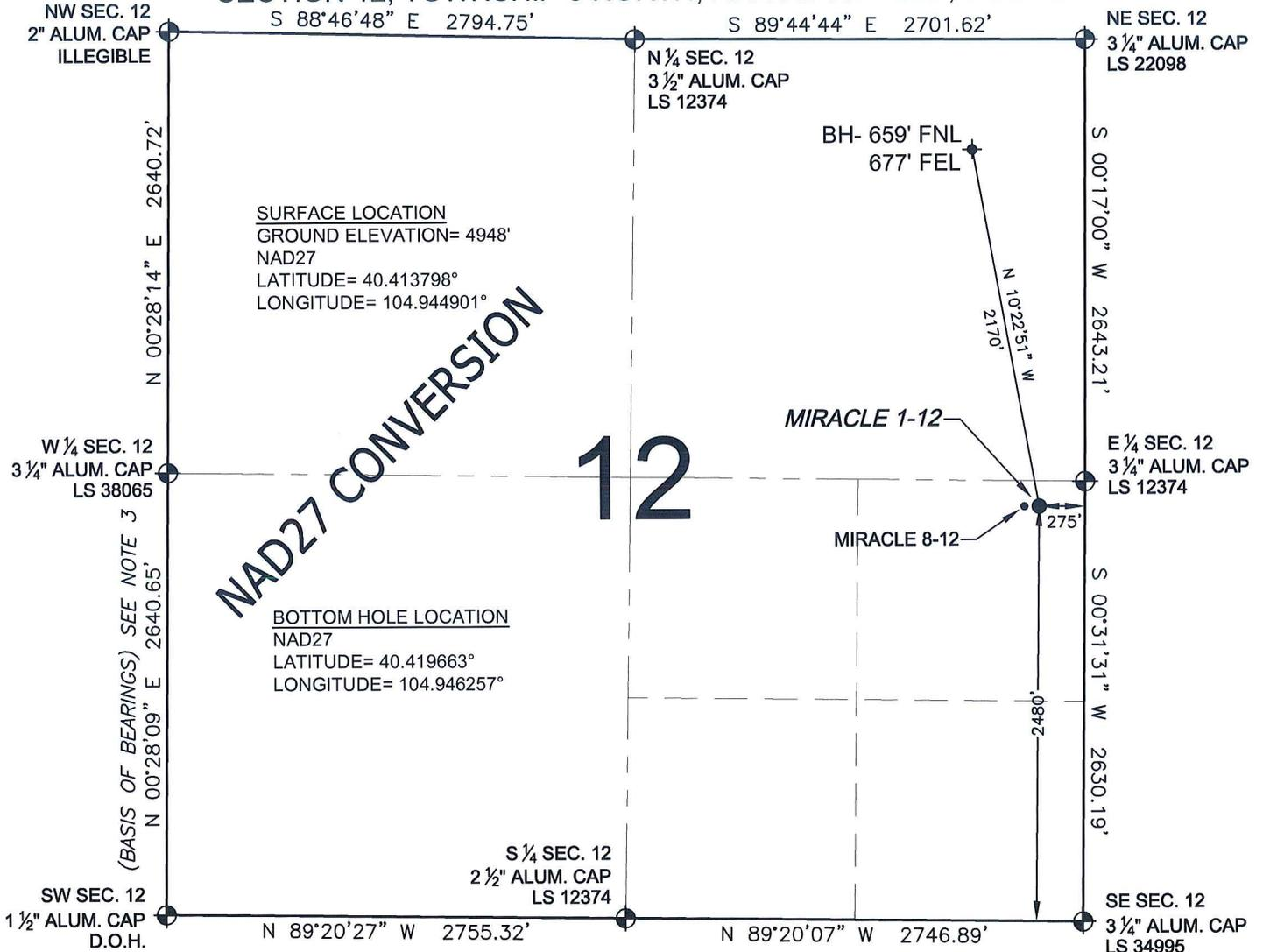
WELL **MIRACLE 1-12** TO BE LOCATED 2480' FSL AND 275' FEL, SECTION 12, T5N, R68W OF THE 6th P.M.
